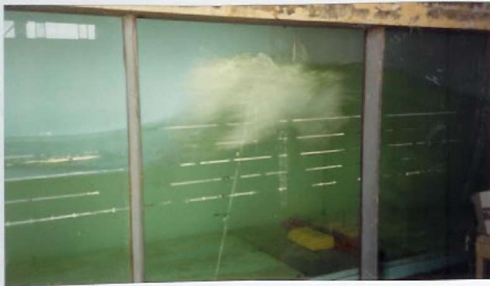
Extreme (breaking wave) Loading of Flexmat/pipes bundle assembly. (Aghincourt Project) Shallow water tests at UWA's major wave flume
