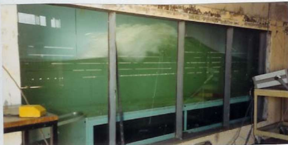
Extreme (breaking wave) Loading of Flexmat/pipes bundle assembly. (Aghincourt Project) Shallow water tests at UWA's major wave flume
