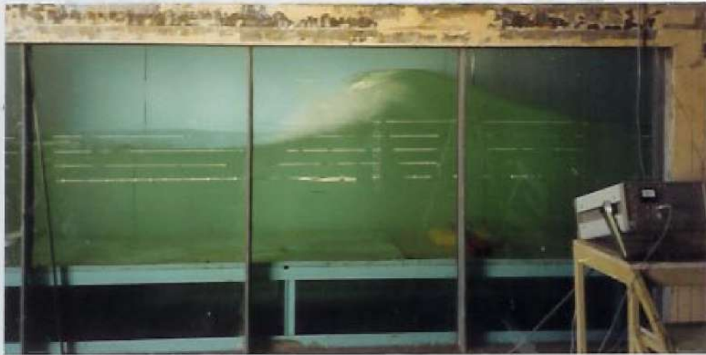
Extreme (breaking wave) Loading of Flexmat/pipes bundle assembly. (Aghincourt Project) Shallow water tests at UWA's major wave flume
